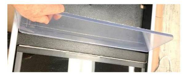
14) Remove the Protective Coating from the Side Shields. Using a 4 mm or 5/32" hex Allen-key to install the Side Shields using the screws provided in the Cash Box. Do not overtighten.
