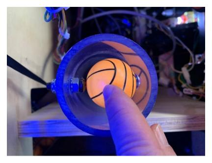
4) Step 4: Adjust the Speed Reducer screw so that the gap between it and the ball is minimal, almost rubbing. Launch a few balls to see how it behaves. Once it's launching properly tighten down the lock nuts on both sides of the chute wall. Try launching a few more balls to make sure.
